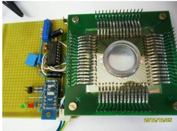
Figure 13 – MEA60 socket and headstage amplifier prototype.
