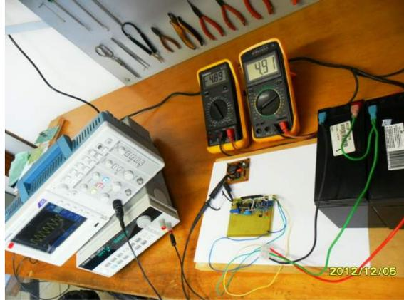
Figure 8 – Headstage amplifier prototype measurement assembly.
